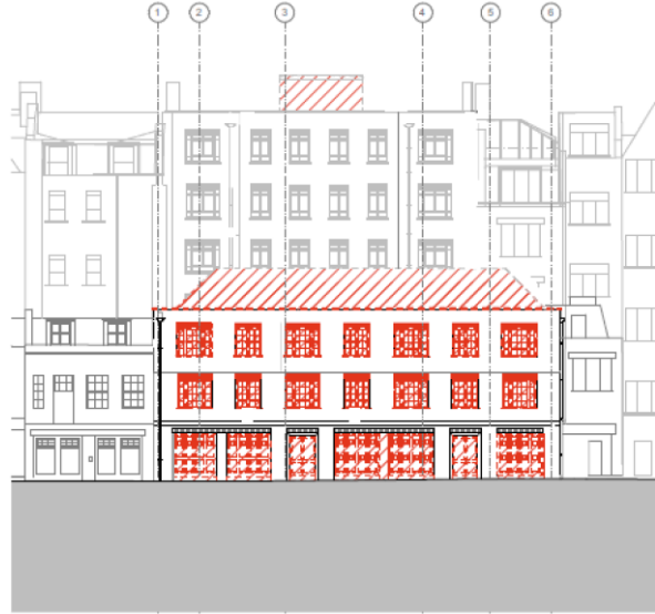
Demolition Harley Place Front Elevation (02)
