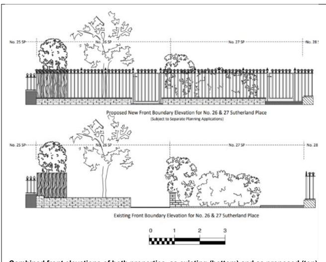
Combined front elevations of both properties, as existing (bottom) and as proposed (top).
